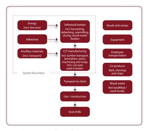
Figure 1: System Boundary and Process Flows
